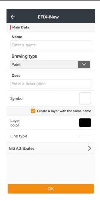
In line survey, if users open **Confirm before saving**, they should give the line name after the start point is measured. In next points, they could name new line name or choose from the existing list before saving it.
