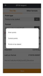
**Format**: user can select the target type from DAT, TXT, CSV, XLSX, and XLS. If the data contains table header, use header should be set by right slide menu.
