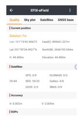
**GNSS base:** Support to view GNSS base status, coordinates, and the distance to the base station.
