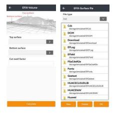
Users can choose surface file or create a new surface file by selecting points. Click **New** to create a new surface file, users can add a new point or select point in **Points**, then click **OK** the interface of "Surface building" will appear.
