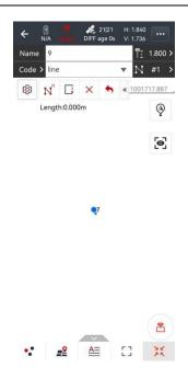
icon opens the line manager. Users could select a line to continue drawing or add a new line. Right slide to get more operations: delete, complete, invert, and rename.
