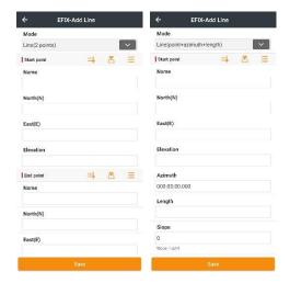
After settings, click **Save** and a line will be created. Users can check the graph by clicking the rectangle button, and inverse the direction by clicking the arrow button.
