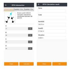
**Points + 2 Sides**: Select points A and B from point management. Enter the length of line AP and line B. Click **OK** to calculate. Input a name, and click **OK** to save.
