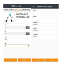
**Points + 2 Angles**: Calculate intersection P with known points A and B and the inner angle of PAB. Click **OK** to calculate. Input a name, and click **OK** to save.
