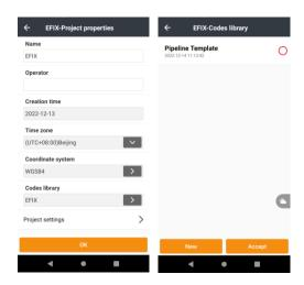
**Pipeline** interface is for surveying pipeline position and collect pipeline attributes. Users will see **Pipeline** icon in menu only after selecting **PIPELINE TEMPLATE** when creating new project.If you can find the **Pipeline** icon ,it can find in **more** .
