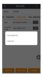
(b) 7 Parameters: Requires at least three known points, and the points can be under the national coordinate system or the coordinate system that existing small rotation from the WGS84 coordinate system. Preferably three or more known points so that eField can check the correctness. The mathematical model of this method is strict, and it is critical to the precision of the known points. This method is usually used in a widerange work.
