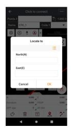
**Off set stakeout point: Users** could manually input coordinates, pick from the map, instant survey, or select from point library. After inputting distance and azimuth, click **Result** then input the **name** of the new point. Click **OK**.
