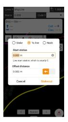
**Node:** The system will automatically choose the spatial point of the polygon or the line. Such as the center of the circle, the corner of the polygon and the line.
