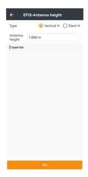
**Vertical H**: The height from ground point to the bottom of receiver. When using range pole, the vertical height is the pole height.
