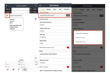
(1) **Survey**: when doing the survey job, you can choose three different survey methods: Topographic point survey, Continuous survey and the Control point survey.
