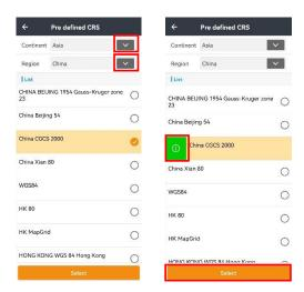
Click **Pre defined** to enter **Common Coordinate** interface, and then users are able to add a new coordinate system by clicking **Selecting**. Slide right and click the green button to check the coordinate system information.
