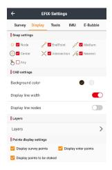
If you want the display of the line width and the line nodes, you can turn these buttons on. When opening a CAD map, you can change the unit and the coordinate system.
