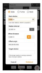
**To line:** Users can stakeout any point on the line in this mode. Users can also change the Start station and the Offset distance.
