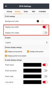
Different layers can be created, and you can choose to display different type of points and change the display of labels.
