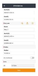
point + azimuth + length + R: Provide the start point, azimuth, length and radius of an arc to create it.
