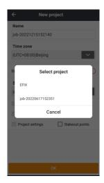
**Note**: Transformation parameters won't be applied if the new project is created without project template. Project template can apply all CRS parameters of the existing project.
