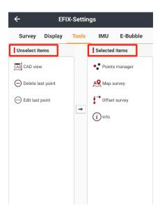
CAD View: Open this data base in the CAD view.
