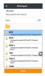
**Note**: After exporting DXF file, you can see shape folder (including .dxf and .shx files) in the same root catalogue of DXF file, please copy both DXF file and shape folder to your computer (must be in the same root catalogue), then correct codes of DXF file will display in your computer.
