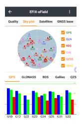
**Satellites**: Support to view the current number of satellites which have been searched, constellation, L1\L2\L5 SNR, elevation angle, azimuth, and locked status.
