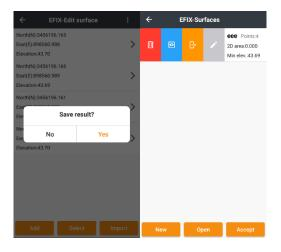
**Open surface File**: Click to open the surface file. Including CASS DTM File, HC DTM File, 3D DXF file and LandXml File.
