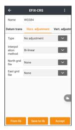
(5) **Vert. adjustment**: Supports four kinds of algorithms: **No adjustment**, **Constant adjustment**, **Surface Fitting** and **Inclined plane**, of which **No adjustment** is the default one.
