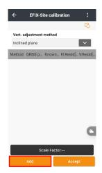
**Vert.adjustment Method**: Include Inclined plane, Constant adjustment, Surface fitting. Default plane fitting method is Inclined plane.
