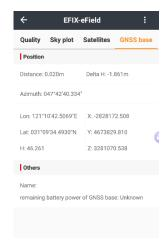
**More:** Click the button on the right side of the interface, the elevation mask and data output frequency setting will show here. Choose Elevation mask setting to set the value and choose Positioning data output frequency to set the RTK update rate.
