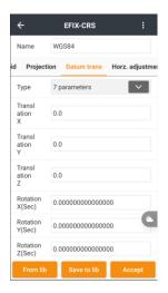
**Note**: When accuracy of known points is not high, 7 parameters transformation is not recommended.
