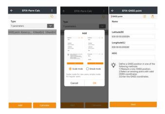
**Note**: Select three corresponding point pairs and add to the interface of parameters calculation.
