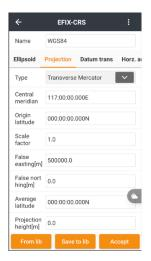
(3) Datum Trans: mathematical model for Represents the transformation between two coordinate systems. Datum transformation model includes no transformation, three parameters, seven parameters, seven parameters(strict), and grid models. Users can input the local 7 parameters directly, no needing the site calibration any more.
