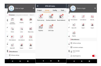
After connecting with pipeline detector, users should use pipeline detector to find target and get pipeline information first. Then, pipeline information can be checked in pop-up window. When there is no problem with pipeline information, users should take away pipeline detector and put receiver on the same position, then click **OK** to survey RTK point. Otherwise, click **Cancel** and detect pipeline again.
