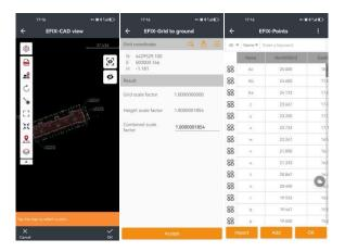
Click **Accept**, and then users will see transformed ground coordinates in point detail. There is no need to apply combined factor when it's 1, because default combined factor is 1 and users can view the ground coordinates in point detail directly. These ground coordinates can also be exported as TXT, DAT, or CSV format with customized content.
