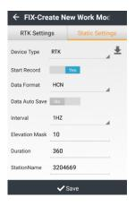
**Interval**: Including choices of 20HZ, 10HZ, 5HZ, 2HZ, 1HZ, 2S, 5S, 10S, 15S, 30S and 1M.
