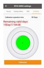
Click to get the offset info of the receiver. When the offset angle is less than the limit value, users can click OK, and then start E-Bubble calibration.
