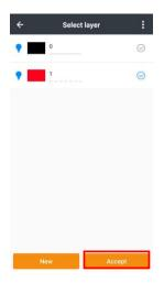
Also they can create a new layer by clicking **New**, then input the layer name and select color and linetypes. Click **OK**, so the new layer would be created.
