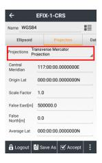
(3) **Datum Trans**: Represents the mathematical model for transformation between two coordinate systems. Datum transformation model includes none parameter, three parameters, seven parameters, seven parameters Bursa, and grid models. Users can input the local 7 parameters directly, no needing the site calibration any more.
