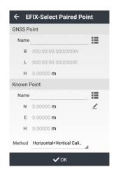
Calculate: Click to calculate. The software will prompt "plane correction success, height fitting success". After that click Application, the prompt is "Whether replace the current project engineering parameters or not", select Yes will make current calculated correction parameters apply in the coordinate system which can affect into the whole project. Users can log for viewing plane correction and elevation fitting parameters, otherwise parameters are not display.
