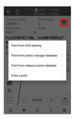
**DIST**: Refer to the horizontal distance between current position and target point.
