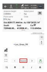
Stakeout **offset point**: Click **multifunctional icon** to open offset point stakeout. Users could manually input coordinates, pick from the map, instant survey, or select from point library. After inputting distance and azimuth, click **Result** then input the **name** of the new point. Click **OK**.
