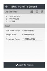
Click **Apply to Project**, and then users will see transformed ground coordinates in point detail. There is no need to apply combined factor when it's 1, because default combined factor is 1 and users can view the ground coordinates in point detail directly. These ground coordinates can also be exported as TXT, DAT or CSV format with customized content.
