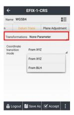
(b) 7 Parameters: Requires at least three known points, and the points can be under the national coordinate system or the coordinate system that existing small rotation from the WGS84 coordinate system. Preferably three or more known points so that eField can check the correctness. The mathematical model of this method is strict, and it is critical to the precision of the known points. This method is usually used in a wide-range work.
