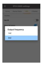
Users can choose to whether "Use tilt" and "Show tilt switch button" or not. Output frequency can be set to 5 or 1 HZ, and the default is 5 HZ.
