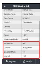
**Note**: Static setting in **Work Mode** is the same as **Static Setting** outside, and the final setting in **Work Mode** or **Static Setting** will take effect.
