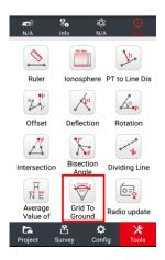
Tap **Grid to** in **Tools** interface. There are three methods to select grid coordinate: from Points, map selection and calculate directly. There needs two points for calculation, the first point coordinates are default as current base station coordinates. Grid scale factor, height scale and combined factor will be calculated after selecting second point coordinates. (Combined factor can also be inputted.)
