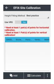
**Height Fitting Method**: Include fixed difference, surface fitting, best practice. Default plane fitting method is best practice.
